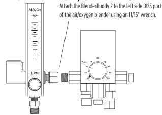
**NOTE:** Low flow BlenderBuddy 2 models (3, 15 and 30 LPM) should only be used with Low Flow blenders. High Flow BlenderBuddy 2 models (70 LPM) should only be used with High Flow blenders. Use outside these applications may result in flowmeter inaccuracies.
