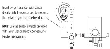
**NOTE:** A small continuous sensor bleed is provided to the analysis port which enables gas analysis regardless of which outlet port is used on the blender.
