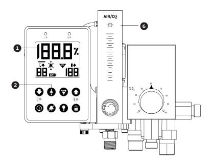
1. Large, Backlit LCD Provides clarity in low-light environments
